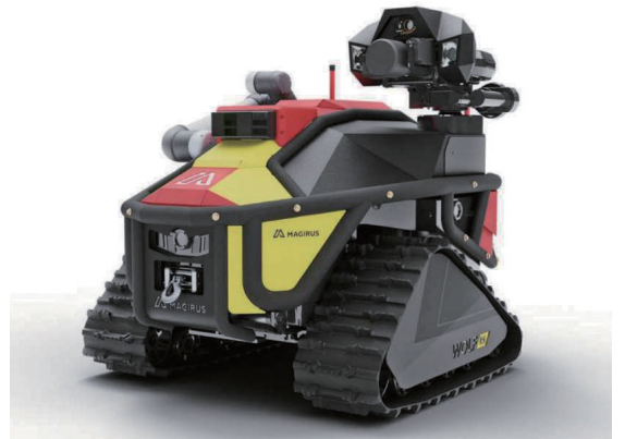
Unmanned water discharge robot
