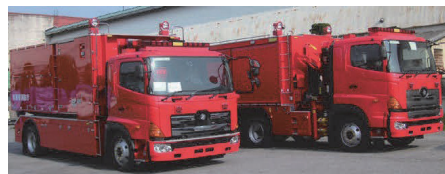
Fire-fighting system using seawater (Super Pumper)
