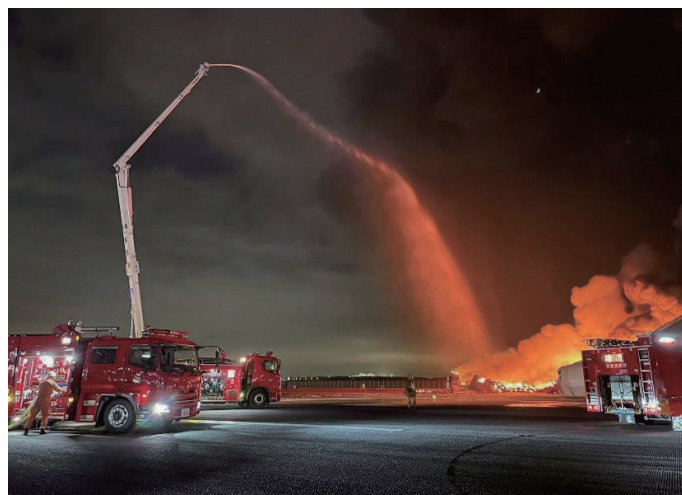
Firefighting using a fire truck with a telescopic water hose (Courtesy of Tokyo fire department)
